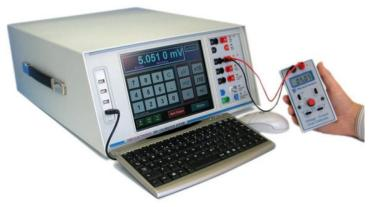
The 5051 is a high performance calibrator combining both source and measure functions. It's outstanding performance is based on Time Electronics own 22 bit Digital to Analogue converter which provides 0.25ppm resolution. The linearity and temperature coefficients are compensated by patented software techniques to provide better than 0.05ppm/°C.
