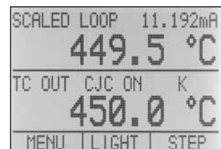
Online scaling, get the difference in the actual unit, saves calculation time and potential errors in the field
