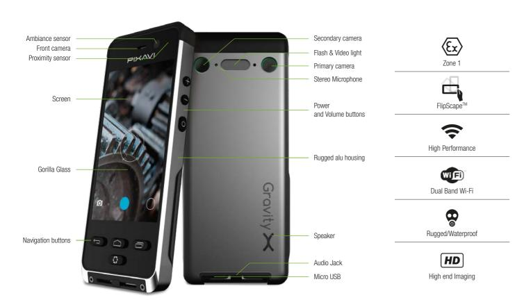
Are you are looking for a lightweight and easy to use HD compact camera for your work in hazardous areas? Using this intrinsically safe digital camera you can also take first-class and high resolution images in places where other cameras may not go.
